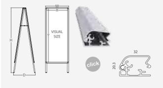
The Poznan A-board frame is made of aluminum so it is lightweight and resistant to rusting and it is available on black or silver color. It has a 32mm width profile with click system, so the graphic change is quick and simple. It includes a weather resistant antireflection protector which allows it to be read under bright lights. Thanks its double-sided frame and its 1800mm height this A-Board is ideal for advertising large offers, menus, information maps, etc, outside or inside your business.
