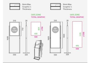
These solid Displays are made of steel and they are black painted, featuring two different graphic size available. Slide the poster (9mm max. thickness) into the groove and display it back-to-back in high traffic areas.
