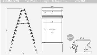
Toulouse double-Sidewalk is made of aluminum so it is lightweight and resistant. It has a 30.5mm width profile with click system, so the graphic change is quick and simple. Also it includes a resistant antireflection protector which allows it to be read under bright lights. Features a headboard support for displaying company logos or graphs. Ideal for displaying sales or promotions at restaurants, stores, shops or supermarkets.
