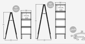
This anodizaded aluminium A-Board is very lightweight, foldable for an easy storage and very resistant to rusting. It features a 25mm width profile with click system, so the graphic change is quick and very simple. Also it includes a weather resistant antireflection protector. The Mota A-Board range features 2 configurations of A3 frames. They are ideal for advertising sales or special promotions inside or outside your business.
