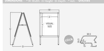
Bayonne Sidewalk is made of aluminum so it is lightweight and resistant to rusting. It has feet protection to avoid slipping and a 30.5mm width profile with click system, so the graphic change is fast and simple. Also, it includes a weather resistant antireflection sheet so is also non-glare which allows it to be read under bright lights. With its 2-sided folding frame, The Bayonne Sidewalk is ideal for advertising sales inside or outside your store.
