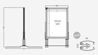
Hervas Sidewalk is made of aluminum and has a strong base with a wide footprint and sturdy springboard design wich allows the flexion in windy conditions. It has a 42mm width profile with click system, so the graphic change is quick and simple. It includes a resistant antireflection protector. Ideal for being used inside or outside your gas station, restaurant, street stall or supermarket for advertising last promotions.
